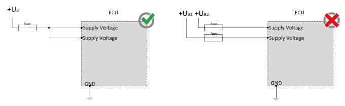
PWM outputs may not be connected with each other or bypassed.
